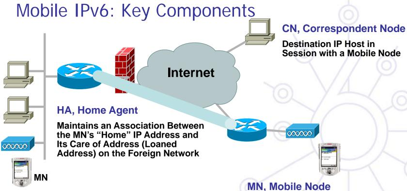
**An IP Host that Maintains Network** Connectivity Using Its "Home" IP Address, Regardless of which Link (or Network) It Is Connected to
