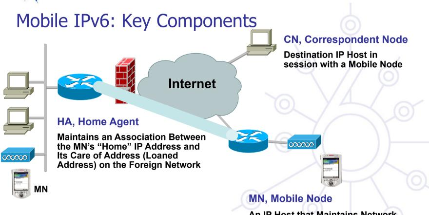
An IP Host that Maintains Network Connectivity Using Its "Home" IP Address, regardless of which link (or network) it Is connected
